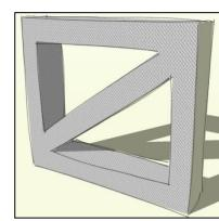
An alternative to triangulation is to use a gusset plate. A gusset is simply a piece of material used to brace and join the members in a structure. A triangular gusset plate has been used here but they can be made in a variety of shapes.
